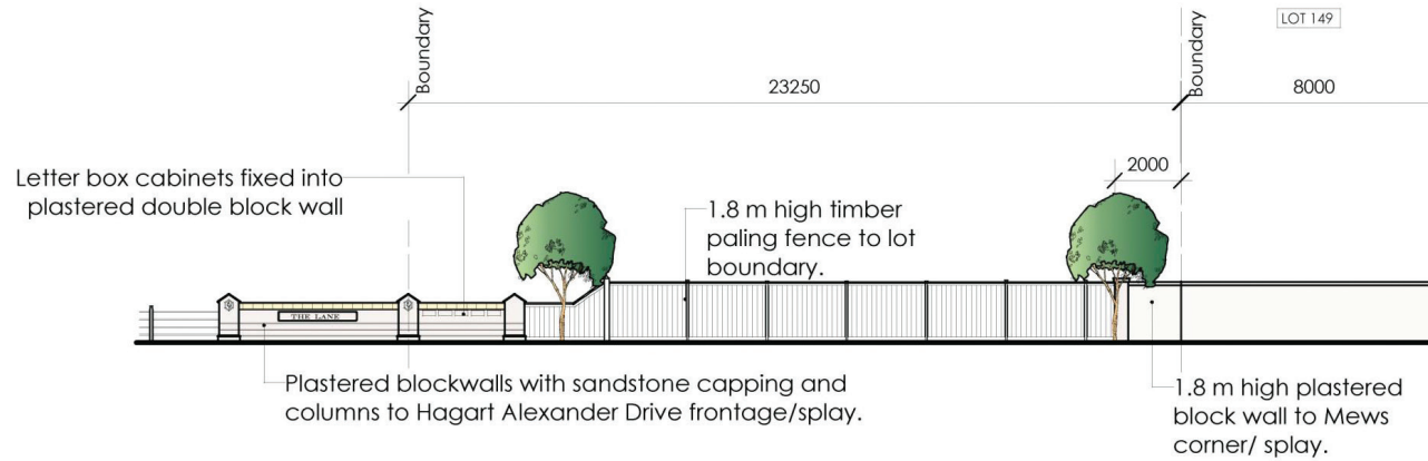
Fig. 7.1 - Developed (part) Elevation - South Elevation Typical Fencing/Walls to Lane Boundaries (Lot 149) Scale: 1:200
